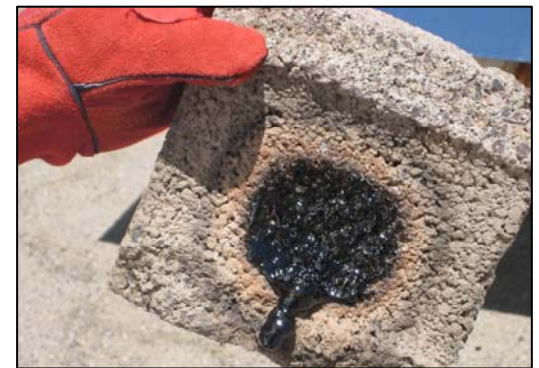
Cinder Block after two minutes in beam
