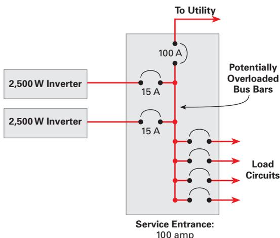
= 10.4 amps. Using the NEC-required 1.25 multiplier (Section 690.8) yields a circuit breaker requirement of 13 amps, which rounds up to 15 amps as the rating of the backfed circuit breaker. On a 100-amp panel, with a 100-amp main circuit breaker, only one of these inverters can be accommodated. On a 200-amp panel, only two of these inverters may be connected, limiting the PV system to 5,000 watts and not the maximum potential of 7,680 watts.
