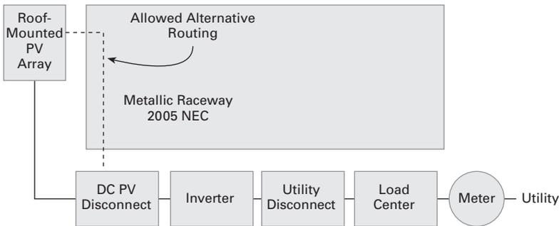
**Fig. 1** shows the simplest configuration of a utility-interactive PV system in which the local jurisdiction requires all disconnects to be located outside the building. In this situation, the AC load center and inverter are also both mounted on the outside of the building.
