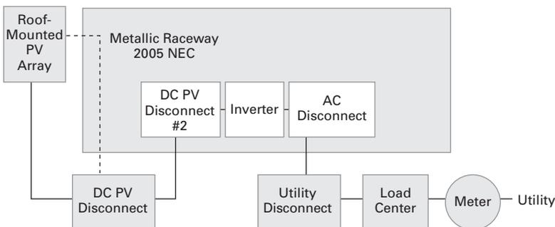
**Fig. 3** reflects situations for which the local jurisdiction requires that the main AC and DC power disconnects (and the main load center containing them) be located outside the building, but for architectural reasons, the inverter be located inside the building. To provide for safe maintenance of the inverter, additional DC and AC maintenance disconnects are needed inside the building at the inverter.
