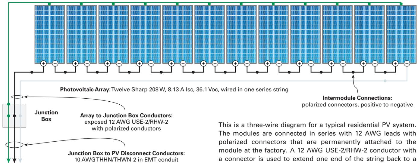
This is a three-wire diagram for a typical residential PV system. The modules are connected in series with 12 AWG leads with polarized connectors that are permanently attached to the module at the factory. A 12 AWG USE-2/RHW-2 conductor with a connector is used to extend one end of the string back to a junction/pull box where it and the other lead are transitioned to 10 AWG THHN/THWN-2 conductors in a  $\frac{3}{4}$ -inch EMT conduit (see *NEC* Section 690.35).
