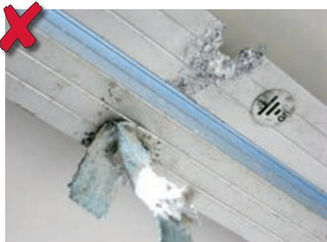
Improper module grounding with dissimilar metals.
