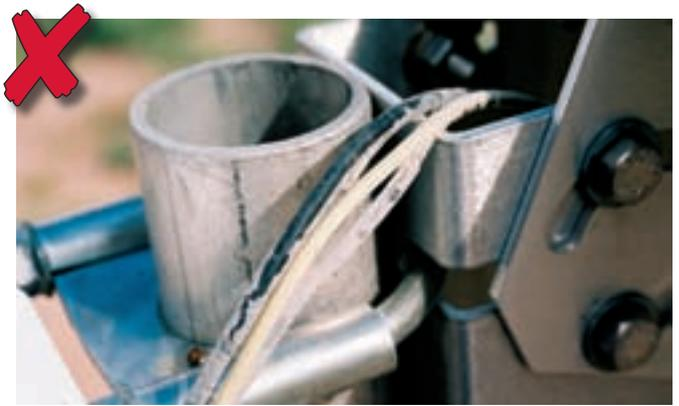
Deterioration of THHN conductors due to outdoor UV exposure.
