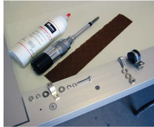
aluminum module frame. Done properly—that is, *with* surface preparation—the presumption is that the mechanical fastener (screw and nut) and the stainless steel washer would carry the fault currents. However, these devices have not been evaluated and listed for carrying current.
