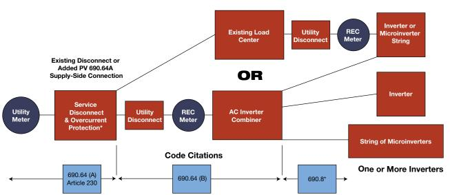
\*Note: If OCPD is installed at inverter, then 690.64(B) applies.
