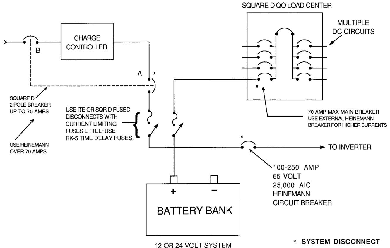
could be isolated from the battery (for servicing) with the fuse disconnect switch if the second pole of the two-pole circuit breaker is not used. The system disconnects must be grouped together so it is probably best to use the two-pole unit because the fuse disconnect switch should be located close to the battery.
