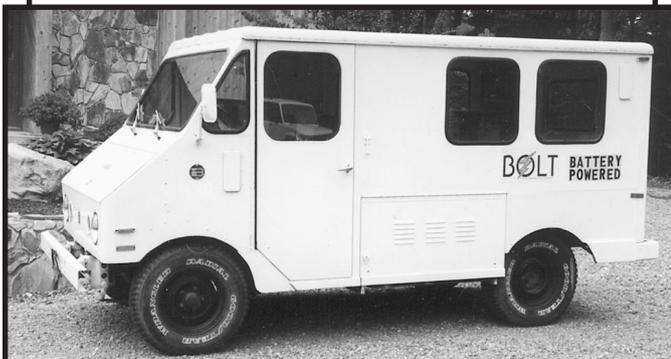
Excellent condition with 1100 actual miles. Perfect for delivery, park, campus, or energy saving events. 112 volt DC 42 HP GE motor, two removable lead-acid tray batteries. Built in battery charger with KWH charging meter, and electronic speed controller. 12 volt lighting, wipers, instruments, gas heater and defroster. \$3500 sale or trade for Trace #SW4024 inverter.
