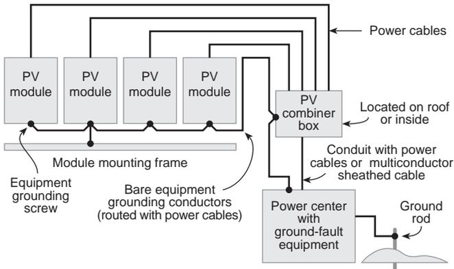
However, smaller conductors are more prone to physical damage and are required to have protection. I suggest #10 AWG (5 mm<sup>2</sup>) as the smallest gauge of bare conductor for equipment-grounding conductors for the exposed wiring to the PV modules. Even this size conductor must be protected from physical damage. In high lightning areas, other equipment-grounding techniques might be used.
