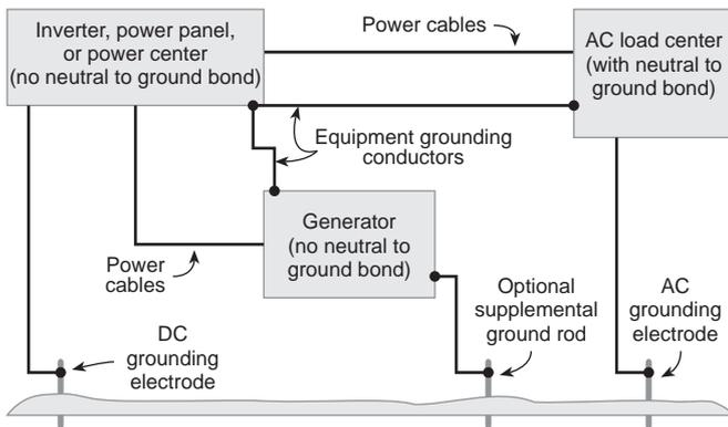
amp circuit will require a #10 AWG (5 mm<sup>2</sup>) equipment-grounding conductor. A 100 amp circuit requires a #8 AWG (8 mm<sup>2</sup>) equipment-grounding conductor. In some locations, a supplemental ground rod may be required for the generator and should be connected only to the generator frame (equipment-grounding system).
