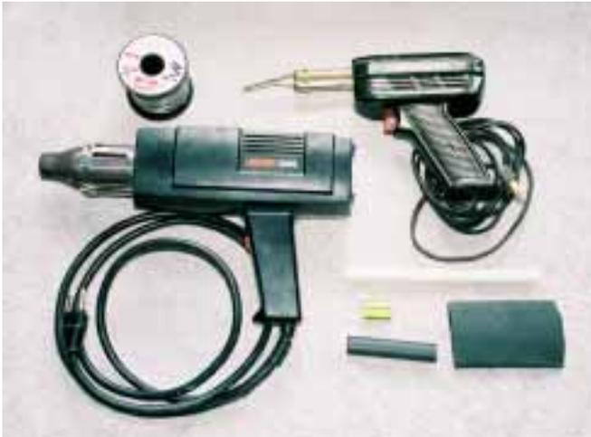
**Use an appropriately sized soldering gun (right) to match your job. A heat gun (left) is used to apply heat shrink tubing to the connection.**
