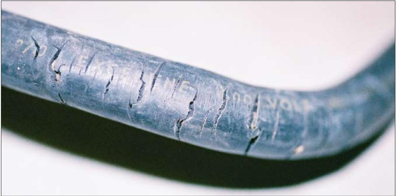
**Photo 5. Improperly specified and sized cable**
