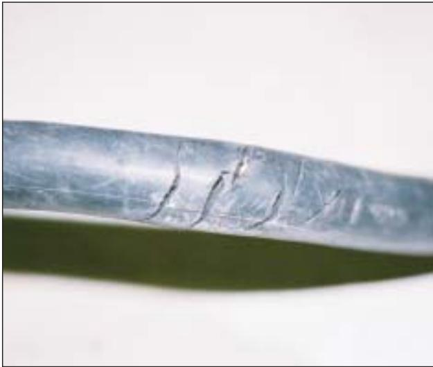
**Photo 8. Welding cable cracked**
