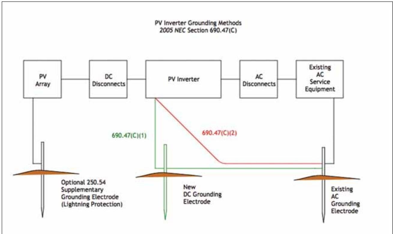
**Figure 1. Grounding small PV inverters per NEC-2005**
