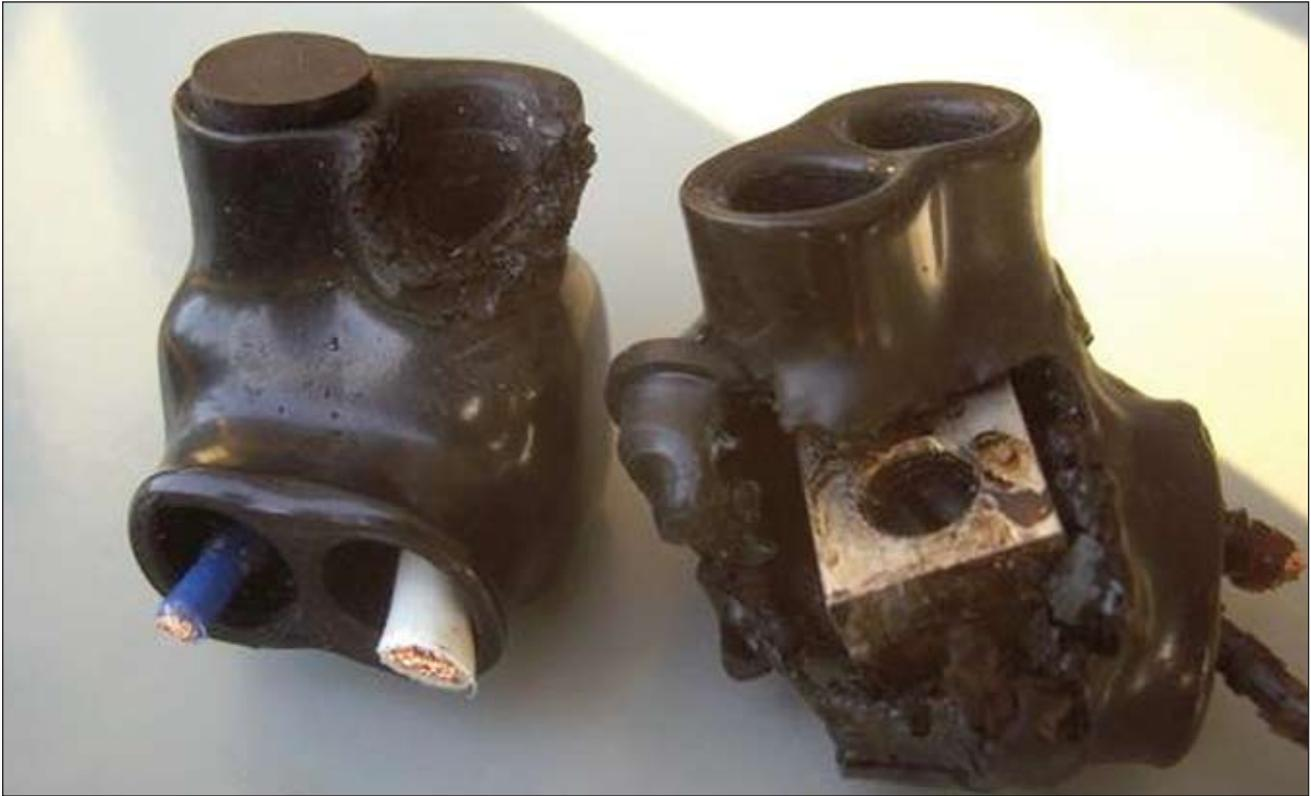
**Photo 6. Improper torque results in failed connections**
