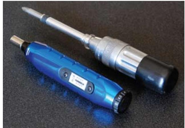
Photo 5. Torque screwdrivers
