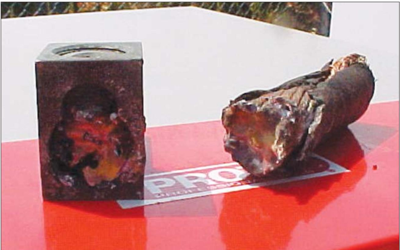
Photo 1. Lug is not suitable for fine-stranded cable.
