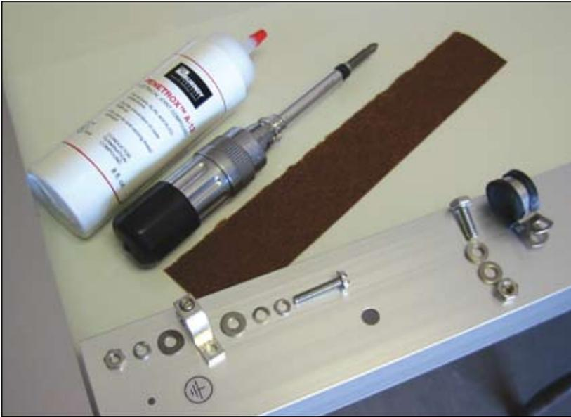
**Photo 3. Module grounding hardware and tools**
