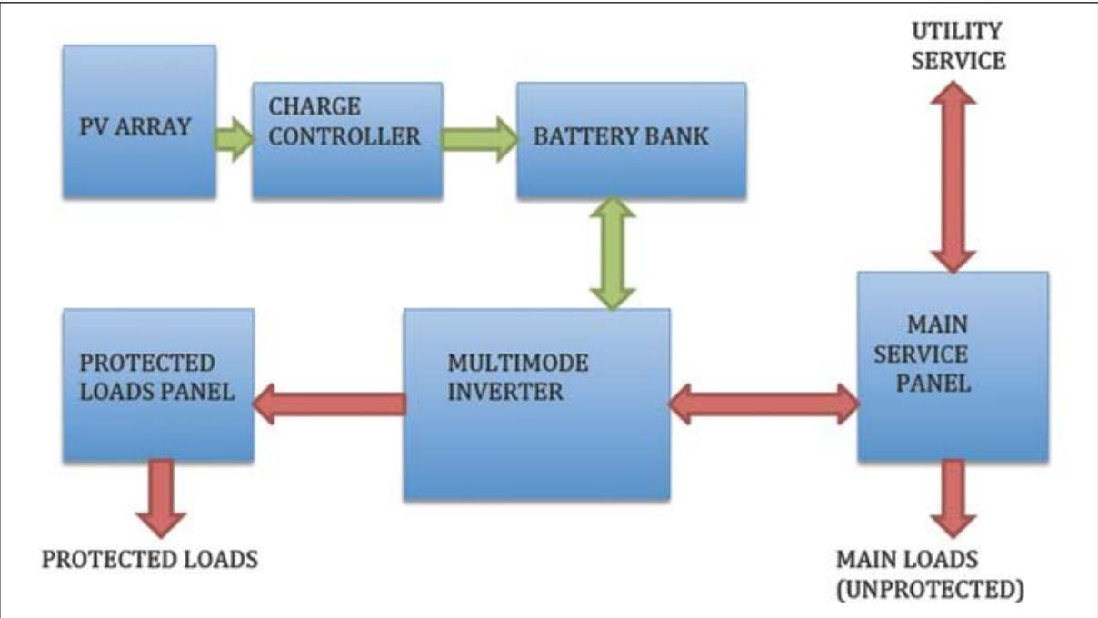
Figure 2. DC-coupled system interconnections and power flows
