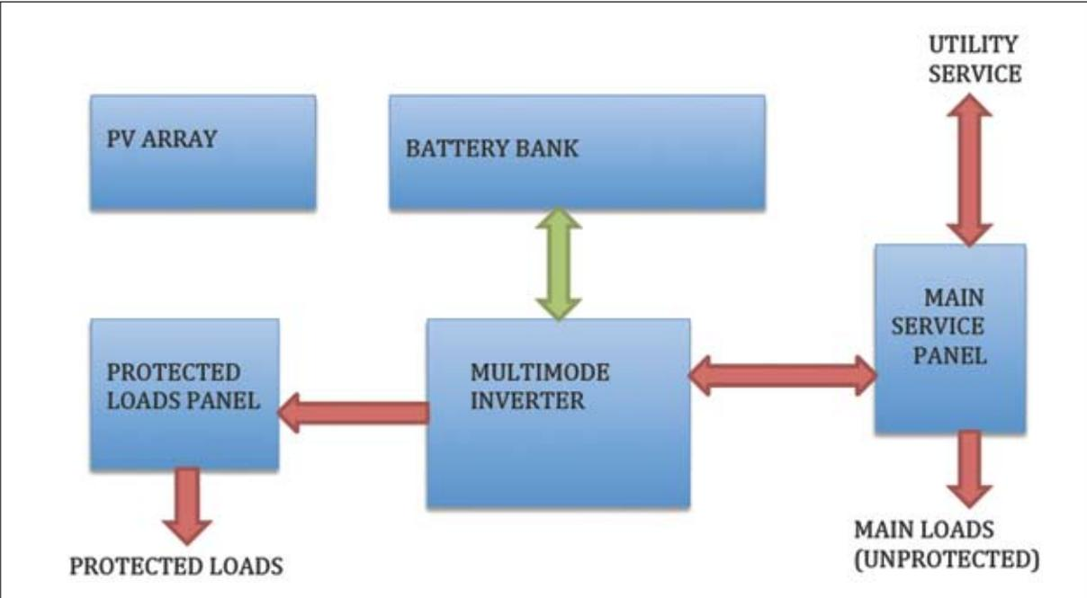
Figure 1. Components in a battery-backed-up, utility interactive PV system
