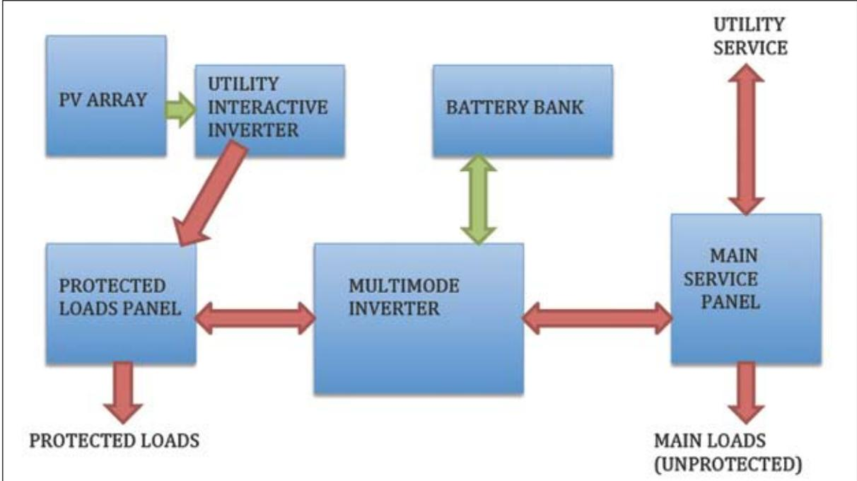
Figure 3. AC-coupled system interconnections and power flows
