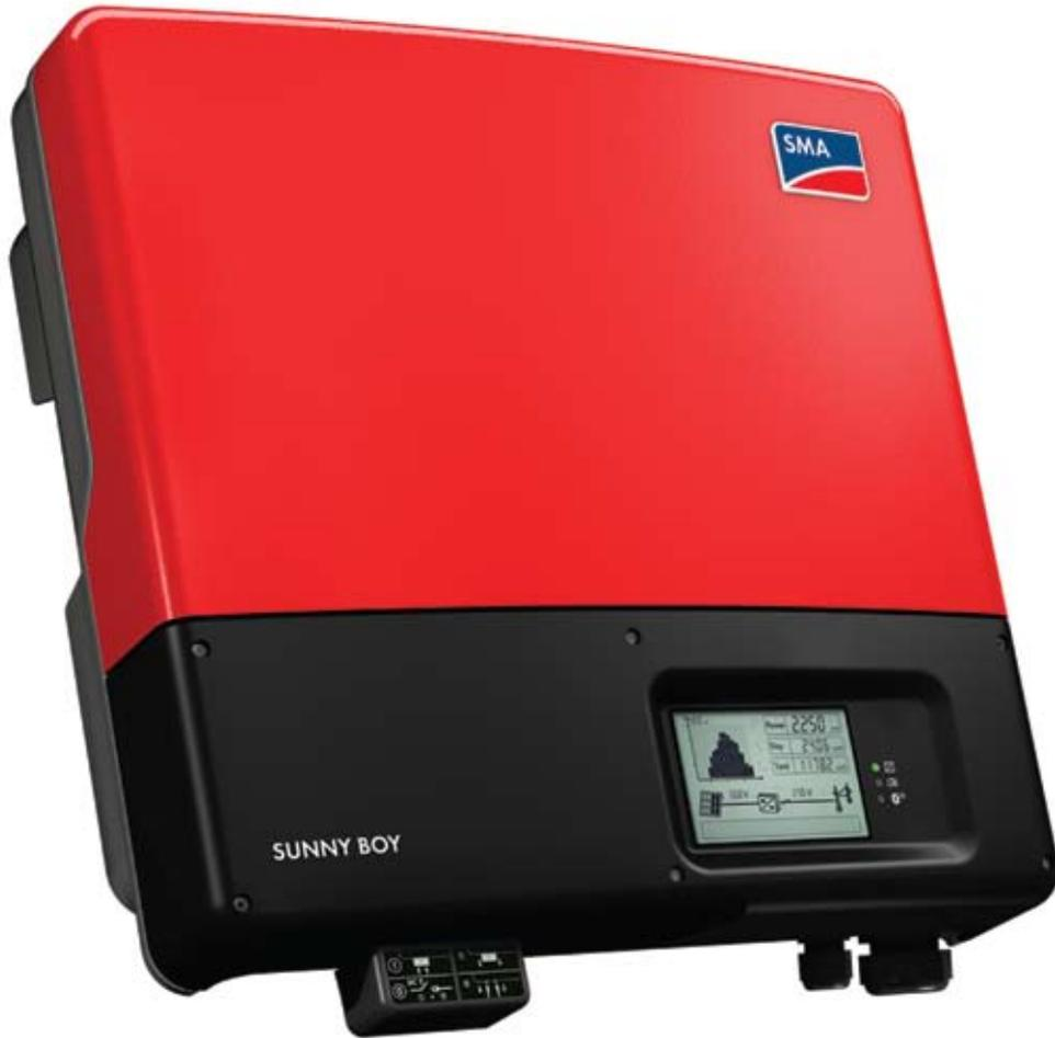
**Photo 1. Transformerless inverter. Looks like many other inverters that have transformers, but may not have a GEC terminal or a 690.5 Warning. Photo courtesy SMA Technologies**
