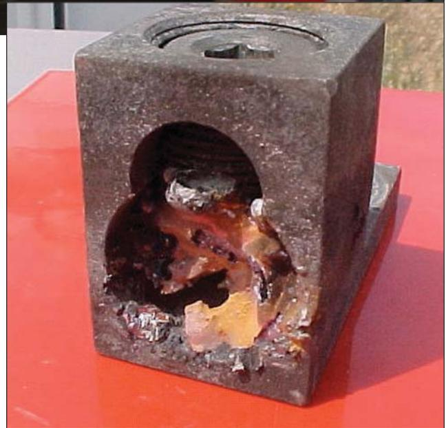
**Photo 5. Fine stranded cable, improperly terminated**
