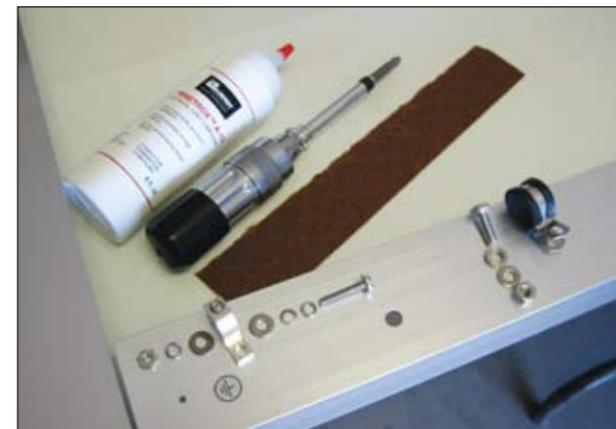
Photo 7. One method of grounding a PV module when all else fails
