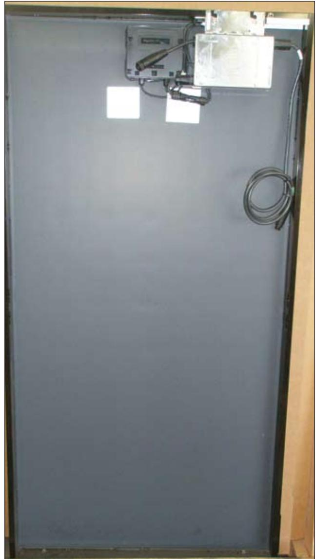
**Photo 1. PV microinverter with exposed dc cables and connectors to PV module**
