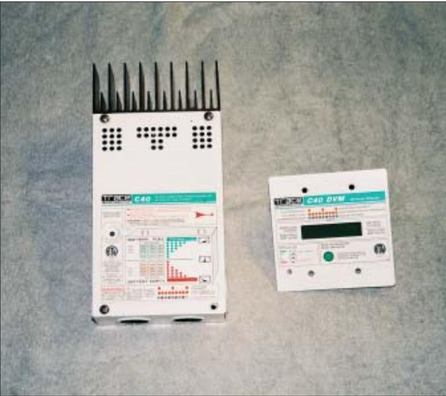
Photo 6. 40 A PV charge controller with remote display
