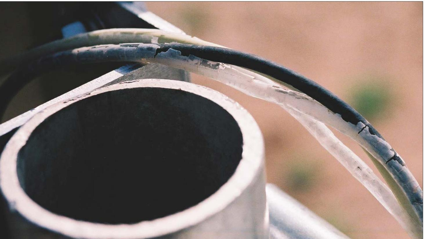
Photo 1. THHN conductors exposed to sunlight
