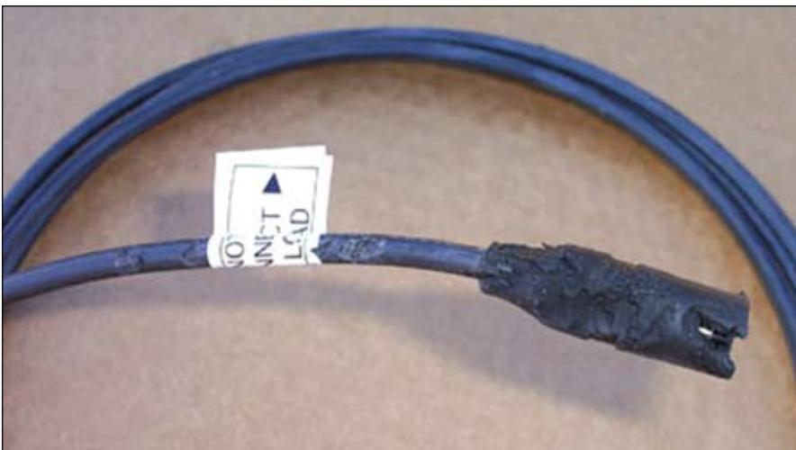
**Photo 4. Rodent damaged cable and connector**
