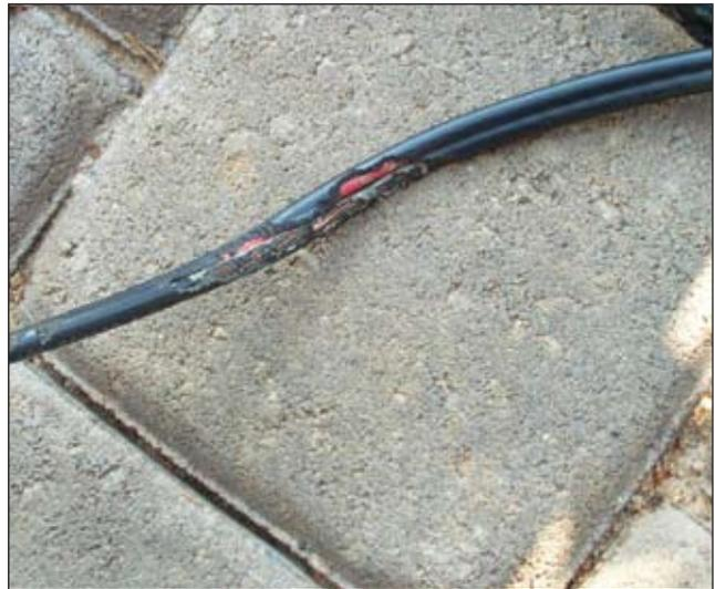
Photo 7. Rodent-damaged conductors
