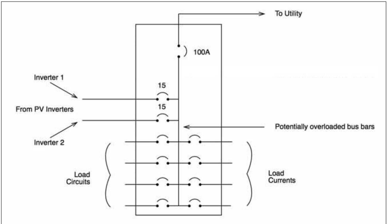
Figure 4. Load-side interconnection diagram
