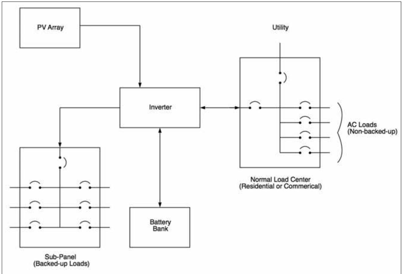
**Figure 8. Utility-interactive PV system with battery backup**
