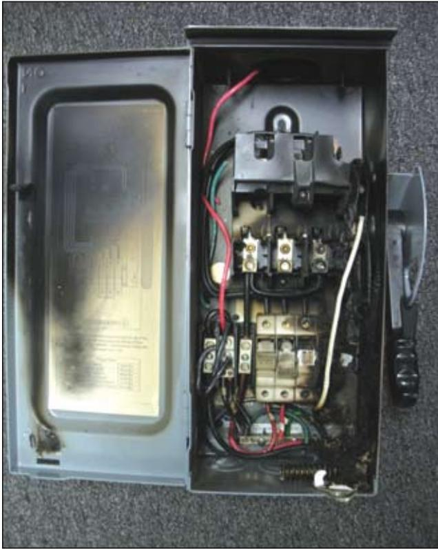
**Photo 1. Burned combiner box caused by wiring error**
