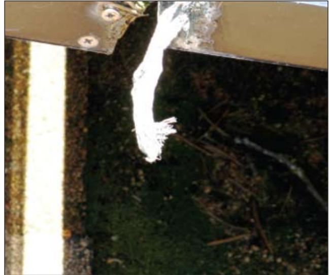
Photo 2. Improper module grounding has failed.
