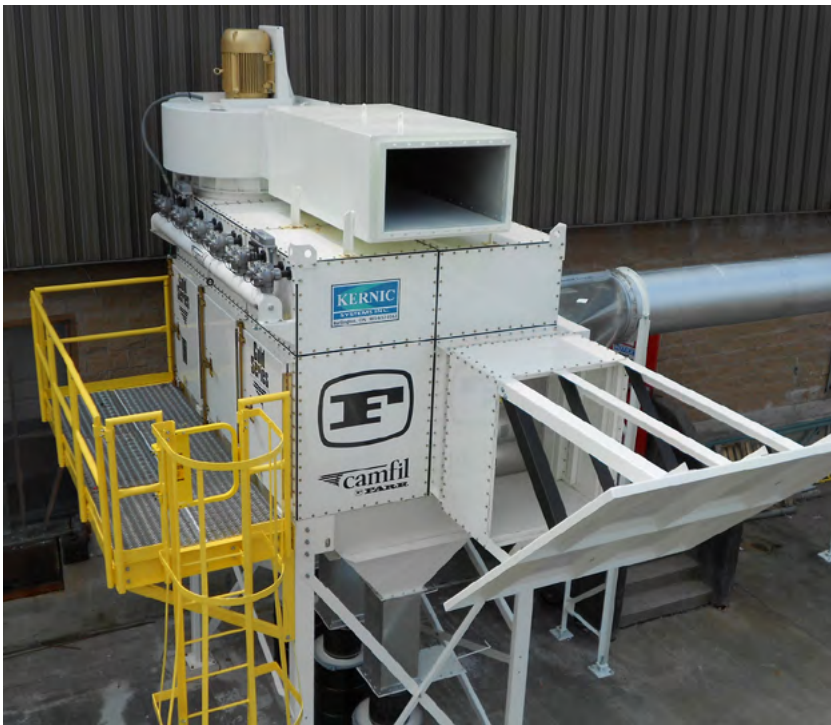
This dust collector is equipped with an explosion vent with vertical upblast deflector plate. Other safety features include a sprinkler system and filters with special carbon-impregnated media for static dissipation.
