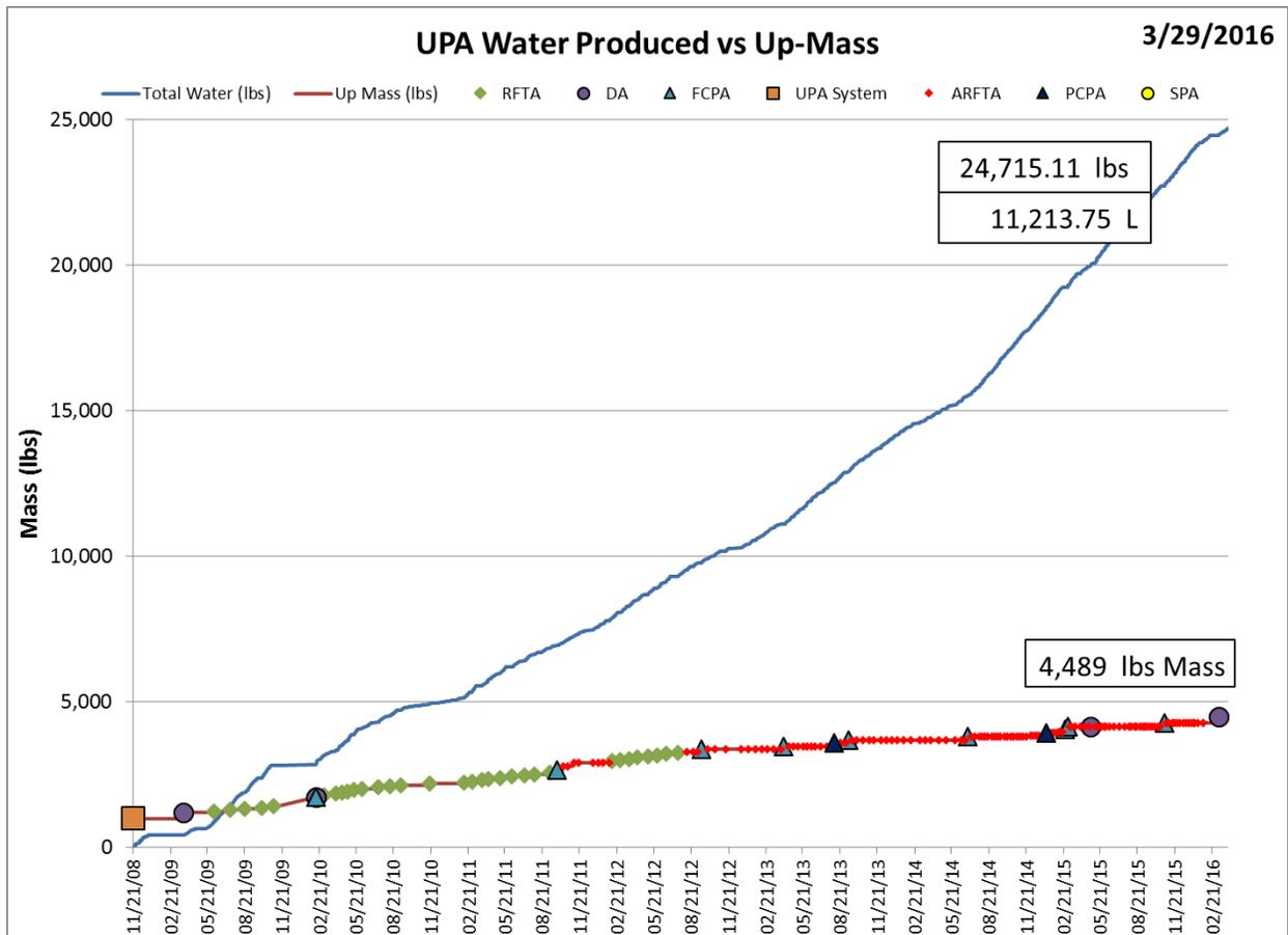
**Figure 5. UPA Production and Upmass on ISS**
