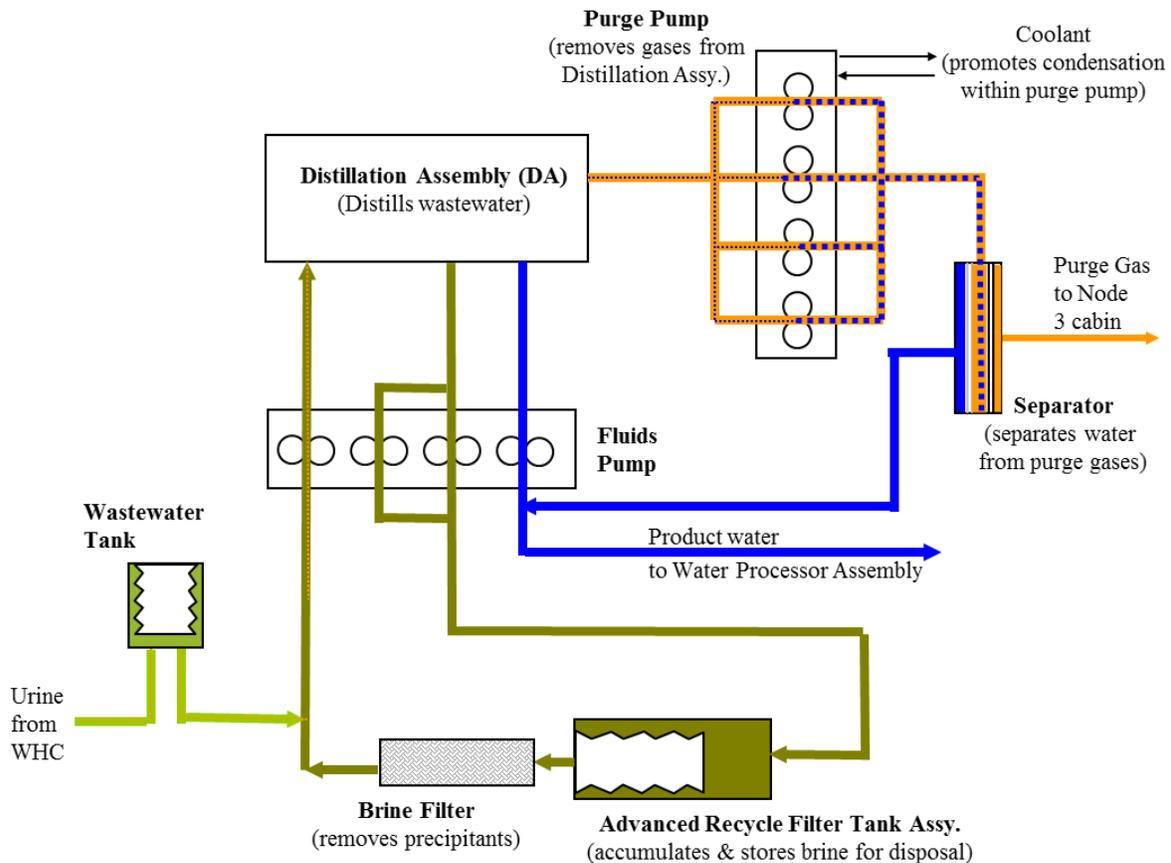
**Figure 4. Urine Processor Assembly Schematic**
