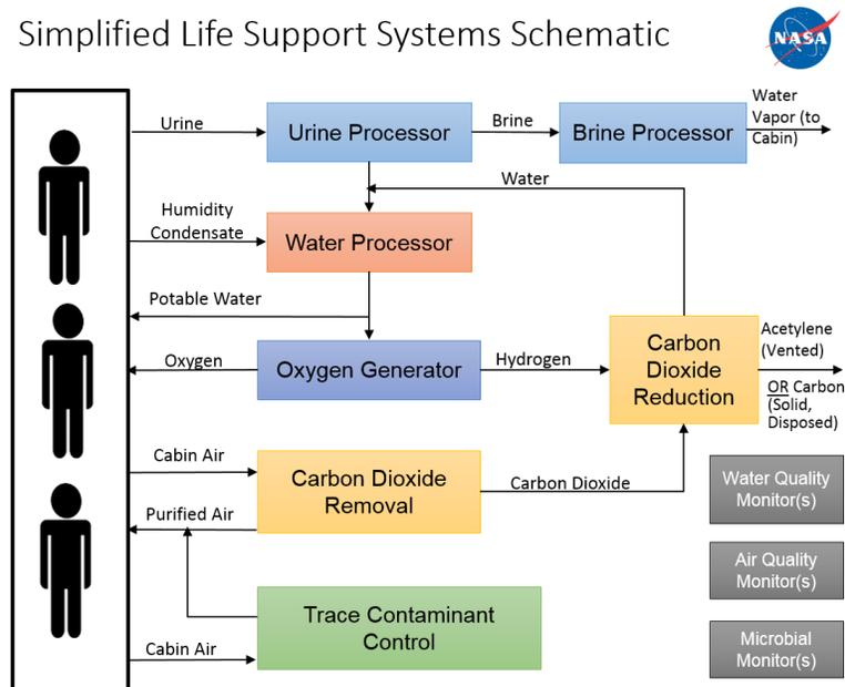
Life support systems schematic for waste, air, and water courtesy of NASA.
